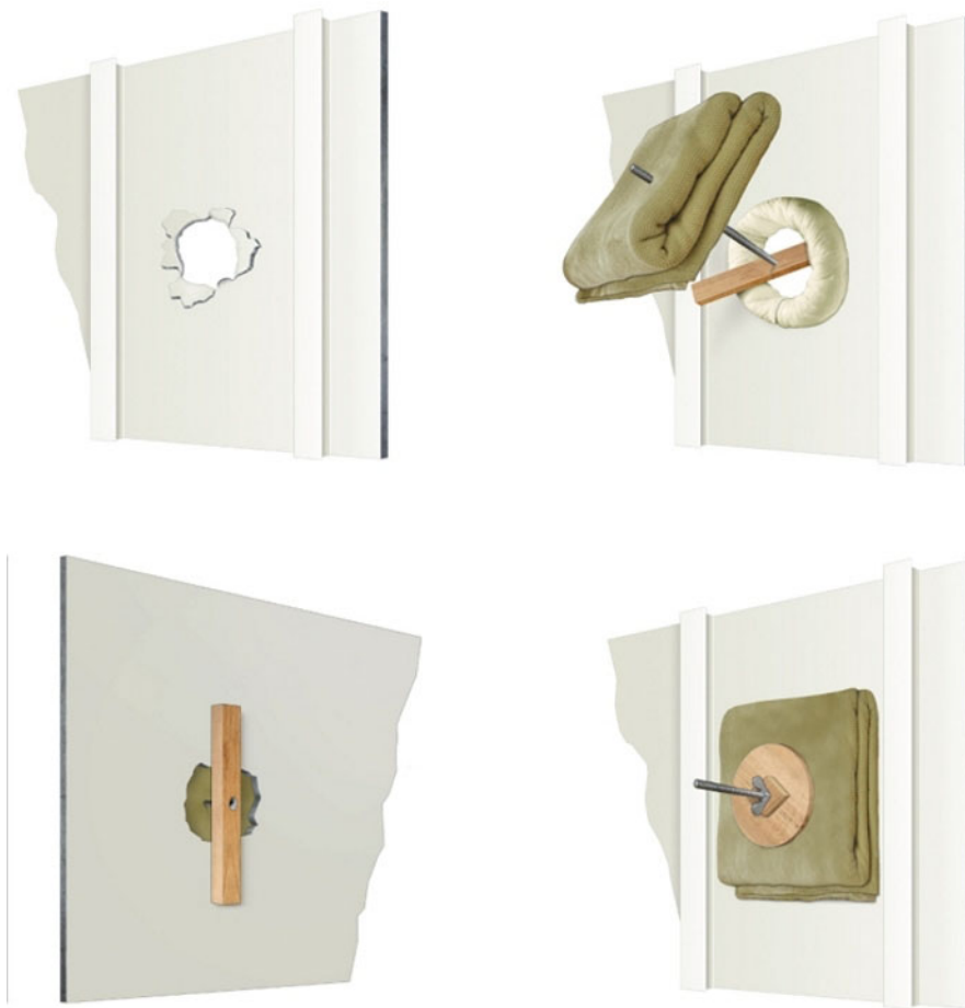
Fig 16-3. Strongback and 'U', 'T' and 'L' Bolts
