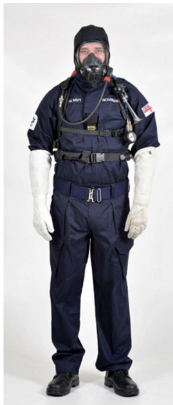
Fig 25-3. Intermediate Firefighting Rig
