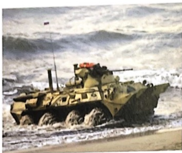
One of the most widely used APCs in the Russian take-over was the amphibious BTR-82 and, as here, the more modern BTR-82A. Widely issued to the Naval Infantry, the BTR-82A mounts a 30mm 2A42 autocannon. (ALEXEY DRUZHININ/AFP via Getty Images)
