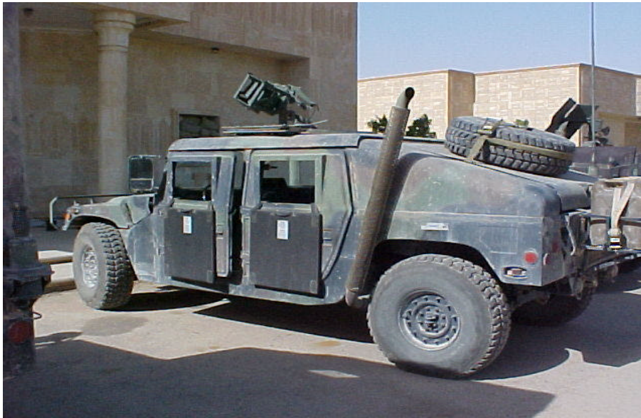
Photo 3-1: SAPI Plate Reinforcement on Doors
