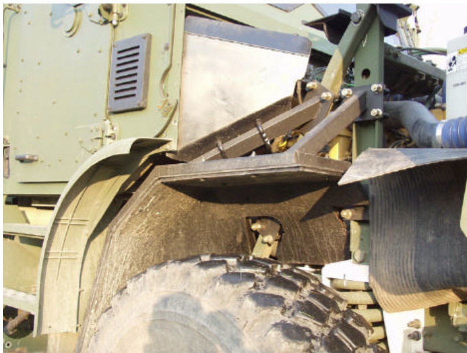
Photo 3-10: Wheel Blast Deflector
