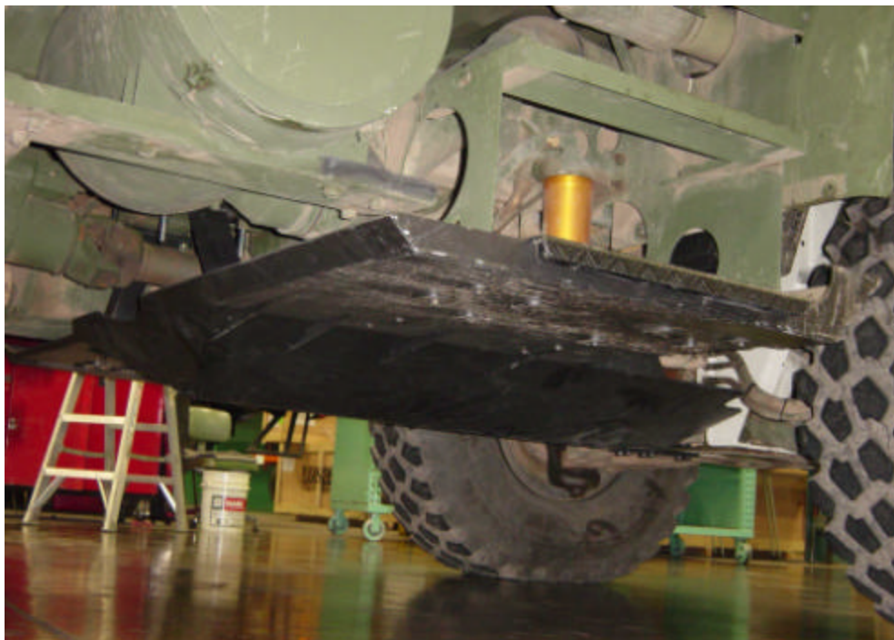
Photo 3-12: Belly Pan Blast Deflector
