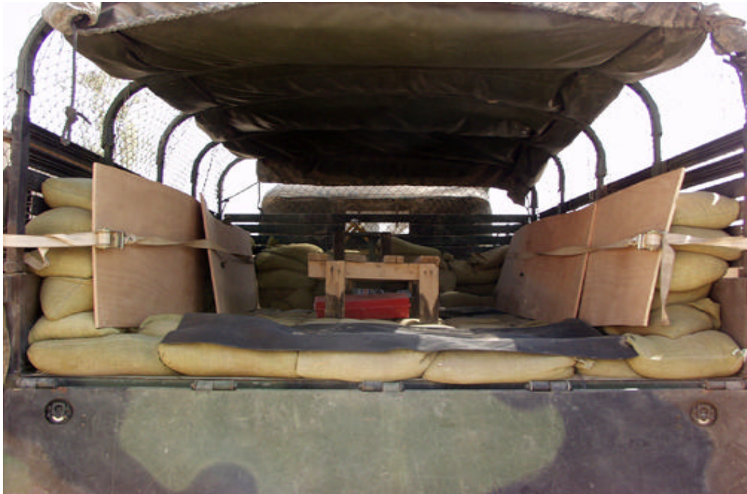
Photo 3-7: MTRV bed reinforced with sandbags and shoring
