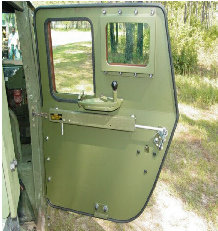
Photo 3-11: HMMWV Marine Armor Kit Door Assembly
