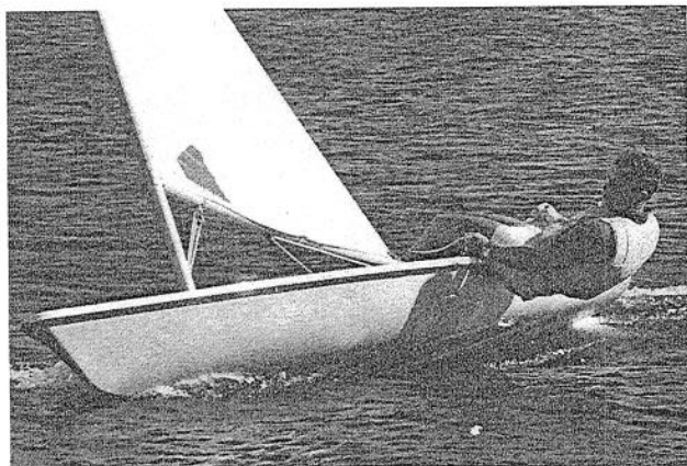
7-13A. Laser roll-tacking sequence. From close-hauled the tiller is pushed to leeward.
