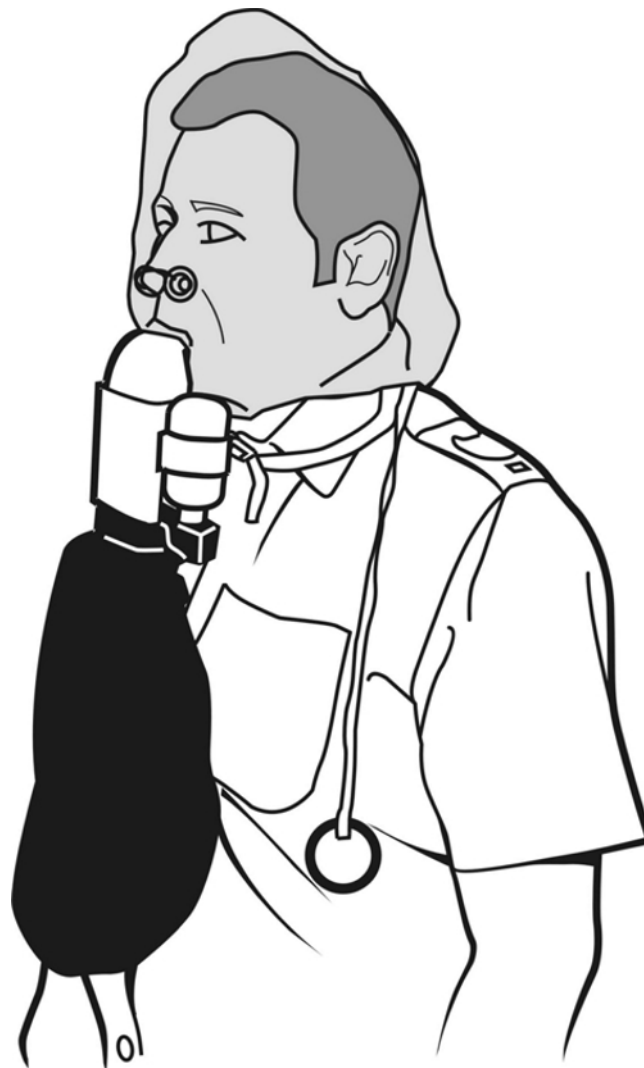
Fig 26-6. Emergency Escape Breathing Device (EEBD)
