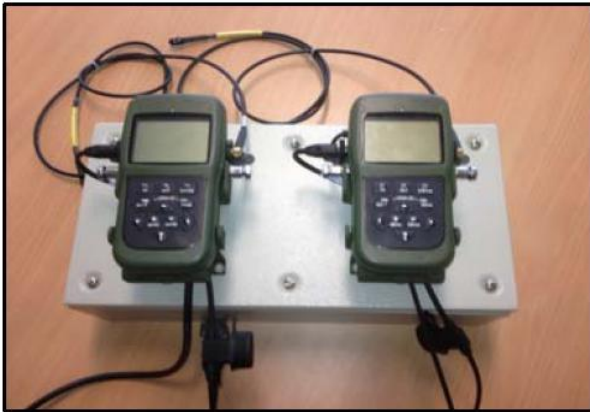
Figure 2-8: FFG DAGR Mounting
