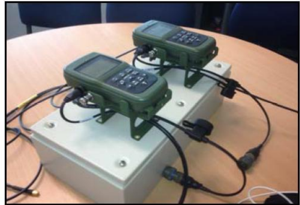
Figure 2-8: FFG DAGR Mounting
