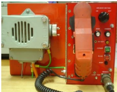
Figure 3-32: ACX-11 Remote Speech Processor
