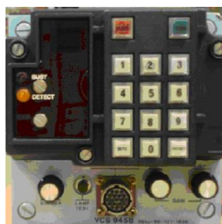
Figure 3-31: VCS-945 Remote Speech Processor
