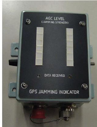
Figure 2-7: GPS Jamming Indicator Unit (JIU)
