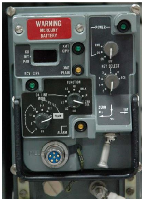
Figure 3-23: ANDVT Voice Crypto
