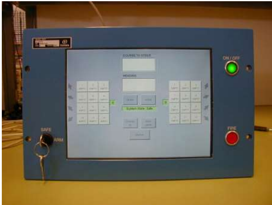
Figure 10-3: SKWS Control Unit
