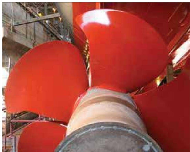
Figure 5: HMS Chatham propeller foul release coating
