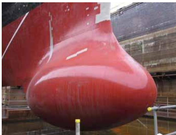
Figure 3: HMS Daring – Foul Release coating after six years in service
