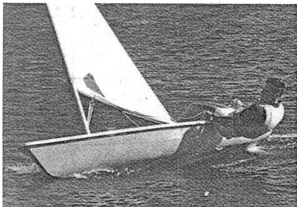
7-15A. Laser roll-jibing sequence. Sailing on a dead run, the boat is heeled to weather as the tiller is put over.
