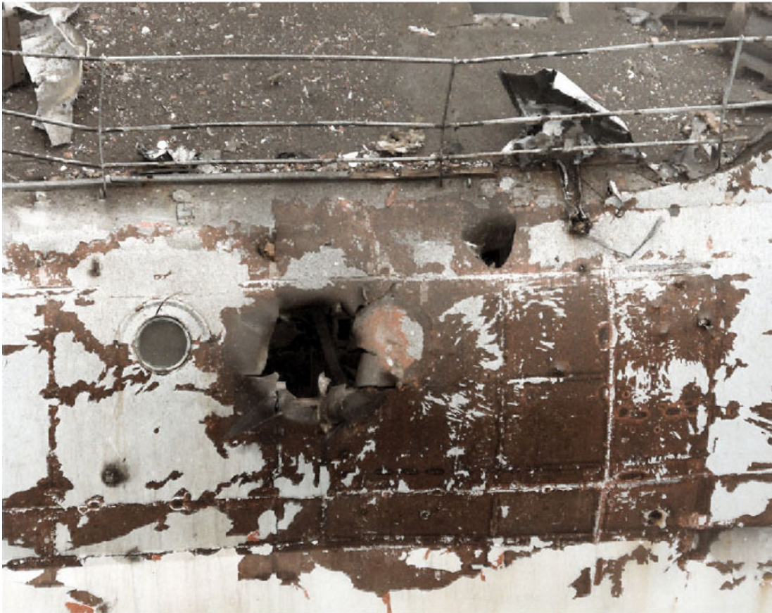
Fig 14-4. Weapon Entry Hole, Showing Petalling of Plating
