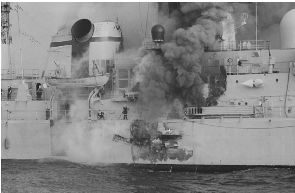
Fig 14-2. Above Waterline Damage Caused by an Anti-Ship Missile
