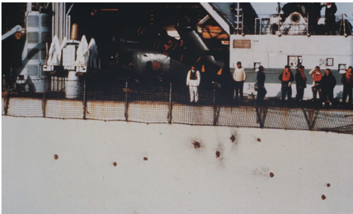
Fig 14-3. Aircraft Cannon Fire Damage
