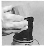
1. Place the focus grip at a slight angle to the Lens Housing and stretch the Grip over the Lens Housing
