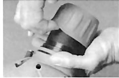
3. Continue pulling the grip up until it disengages from the Lens Assembly
