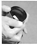
1. Place the focus grip at a slight angle to the Lens Housing and stretch the Grip over the Lens Housing
