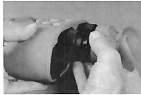
3. Place the eyecup at a slight angle to the eyepiece. Push it toward the eyepiece and rotate to seat it on the eyecup retainer ring
