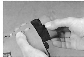
3. Place the eyecup at a slight angle to the eyepiece. Push it toward the eyepiece and rotate to seat it on the eyecup retainer ring
